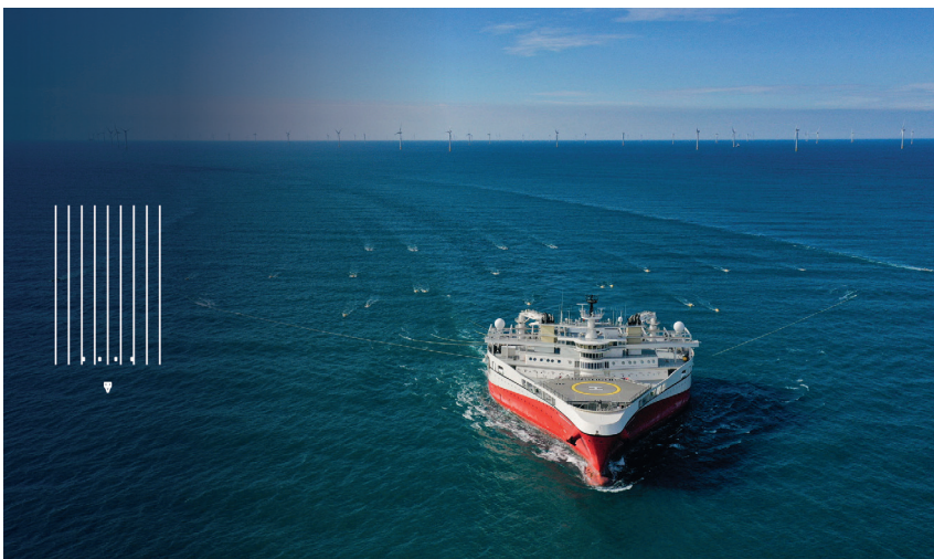
Figure 5 Schematic illustration of the nominal vessel configuration and a photo of Ramform Hyperion acquiring the high-resolution CCS development survey for the Northern Endurance Partnership offshore UK in 2022. The configuration consisted of nine multisensor streamers with 50 m separation and a wide-tow quad source that was towed over the front end of the streamer spread. The resulting nominal acquisition bin size was 6.25 m x 6.25 m.
